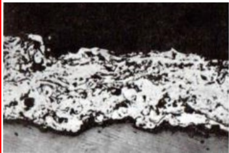
Fig-1. Zinc Sprayed Coating on Grit Blasted Steel
