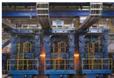
[Section Mill- Break down stand & Compact stand group of CCS design]
