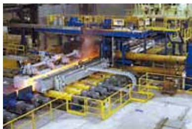
[Section Mill- Break down stand & Compact stand group of CCS design]
