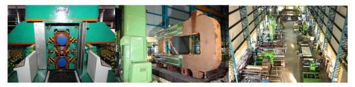
A few of facilities available are Floor & Table type Horizontal Boring Machines, Plano Miller with four functional heads, Bed type Milling Machine, Bed type CNC Milling Machine, Moving Column Milling Machine,
