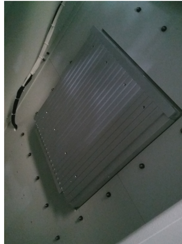
Drive manifold: oil circulating inside it for cooling the drive
