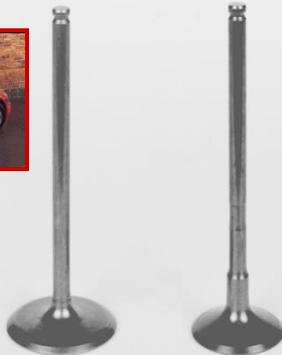
***Ti/TiB for Intake and Exhaust Valves in Toyota Altezza***
