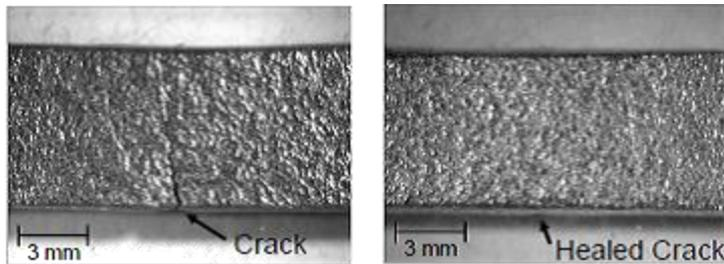
To heal the matrix heat is applied on the surface. Then the SMA nano-fibers recover their original shape sealing the crack. The figure shows how the crack was healed after the heat treatment.
