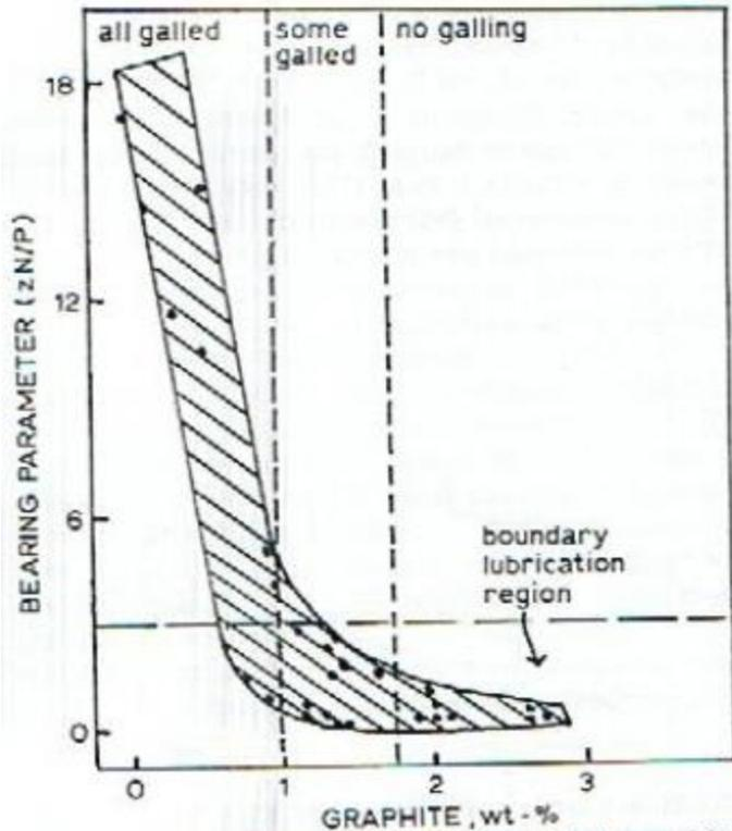
15 Variation of bearing parameter with graphite content for Al-Si alloy base composites
