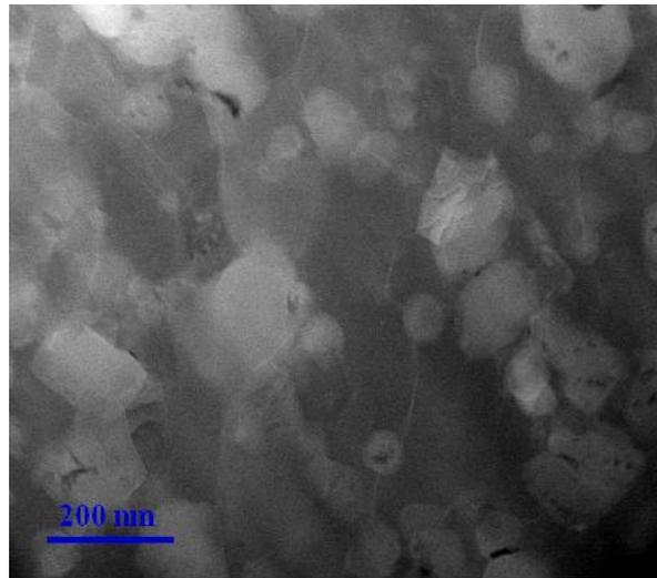
Figure 1. Powder metallurgy based Aluminum alloy-15 vol% Al<sub>2</sub>O<sub>3</sub> [1]
