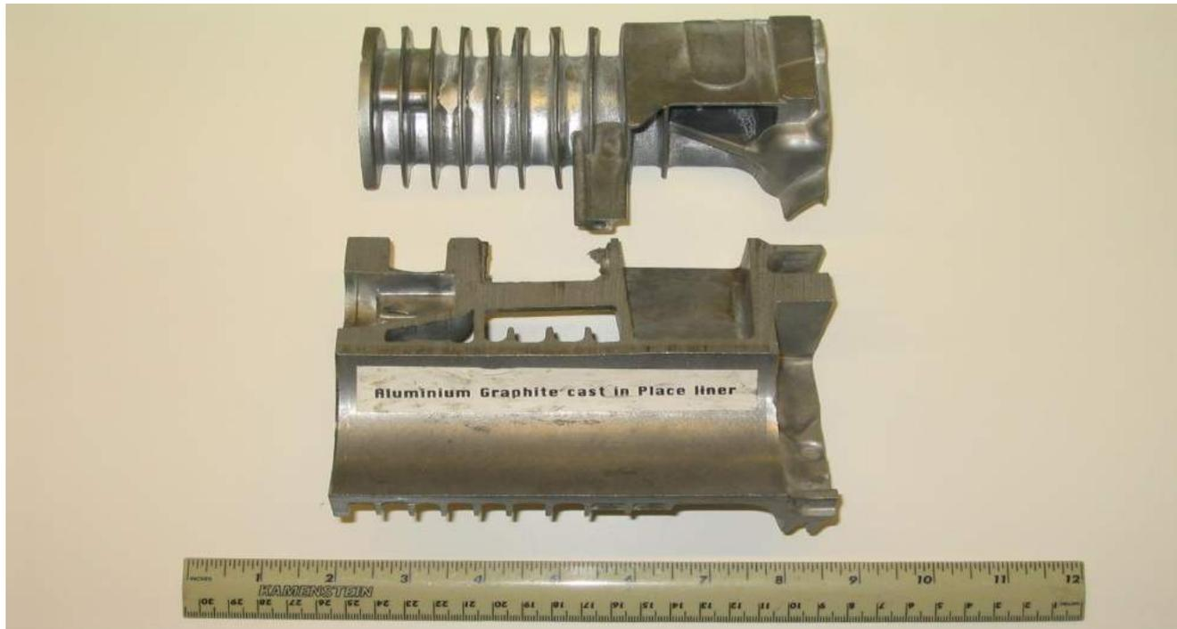
Aluminum Graphite Cast in Place Liner
