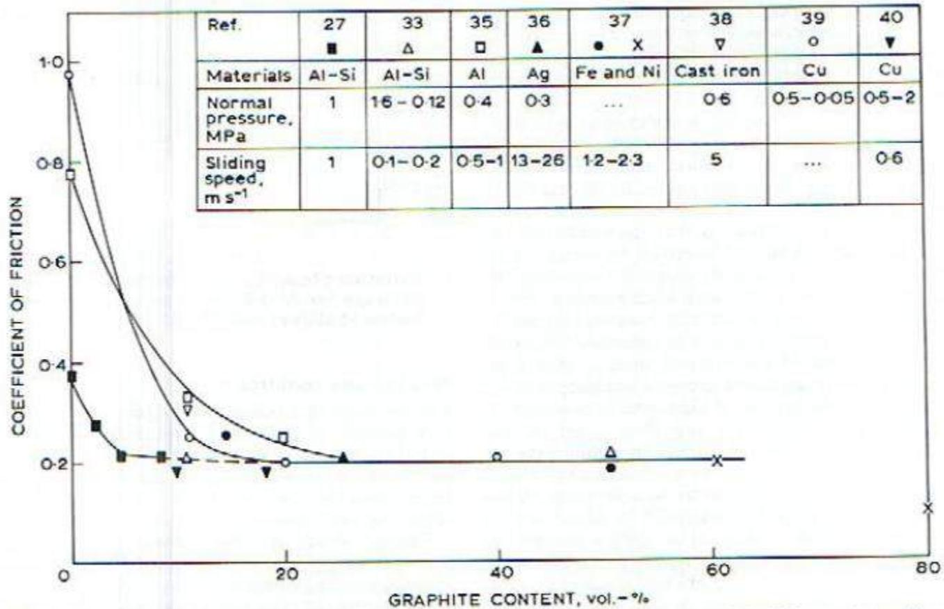
3 Variation of coefficient of friction with graphite content for composites with different base alloys
