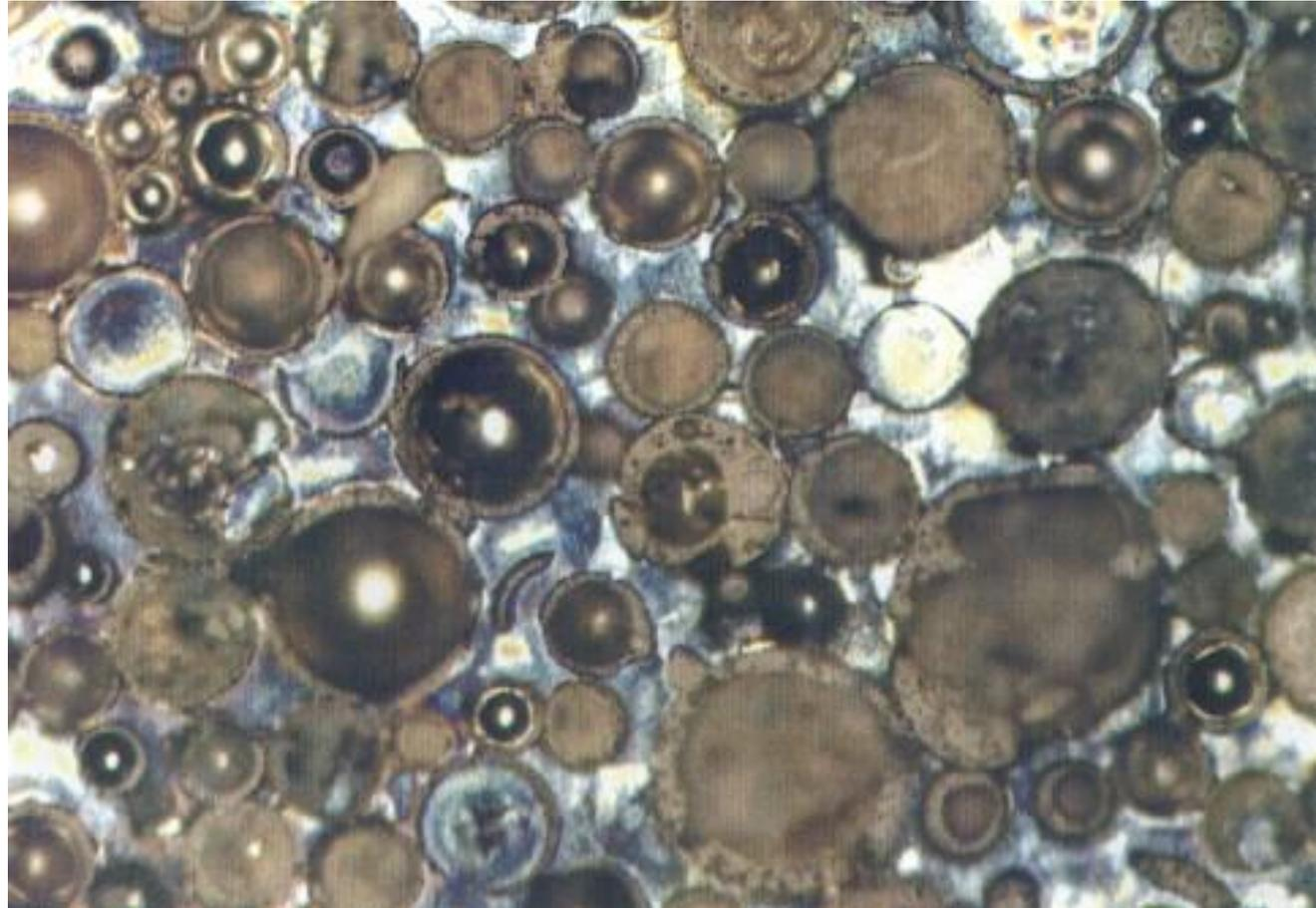
Hollow Fly Ash cenospheres dispersed in the matrix of lead to reduce density
