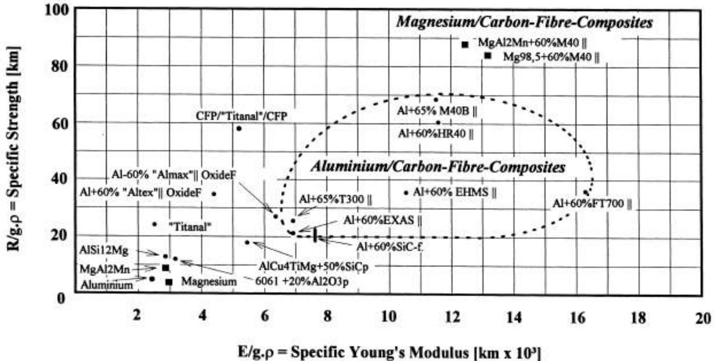
Figure 4 Comparison of specific properties of aluminium and magnesium matrix composites<sup>11</sup> indicating the increase of stiffness and strength with respect to the matrix (longitudinal CFRM properties)
