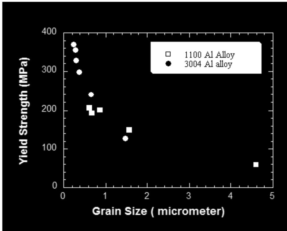
In low alloyed metals strength depends significantly on grain size.
