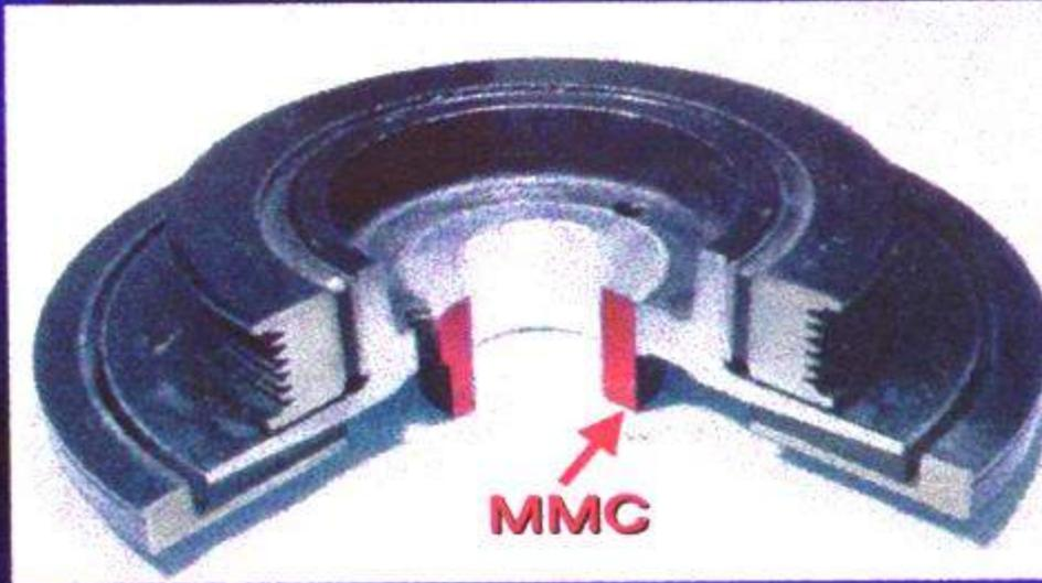
Cut Model of Crankshaft Pulley
