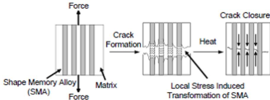
This figure shows the process of healing. The local stress induced by the crack transforms SMA to a Martensite phase.
