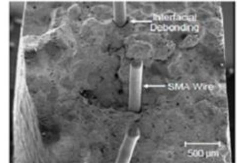
Shape Memory Alloy (SMA) wires in micro size TiNi as the reinforcements, the figure shows the microstructure of the alloy matrix reinforced with Nitinol fibers in micro-scale.
