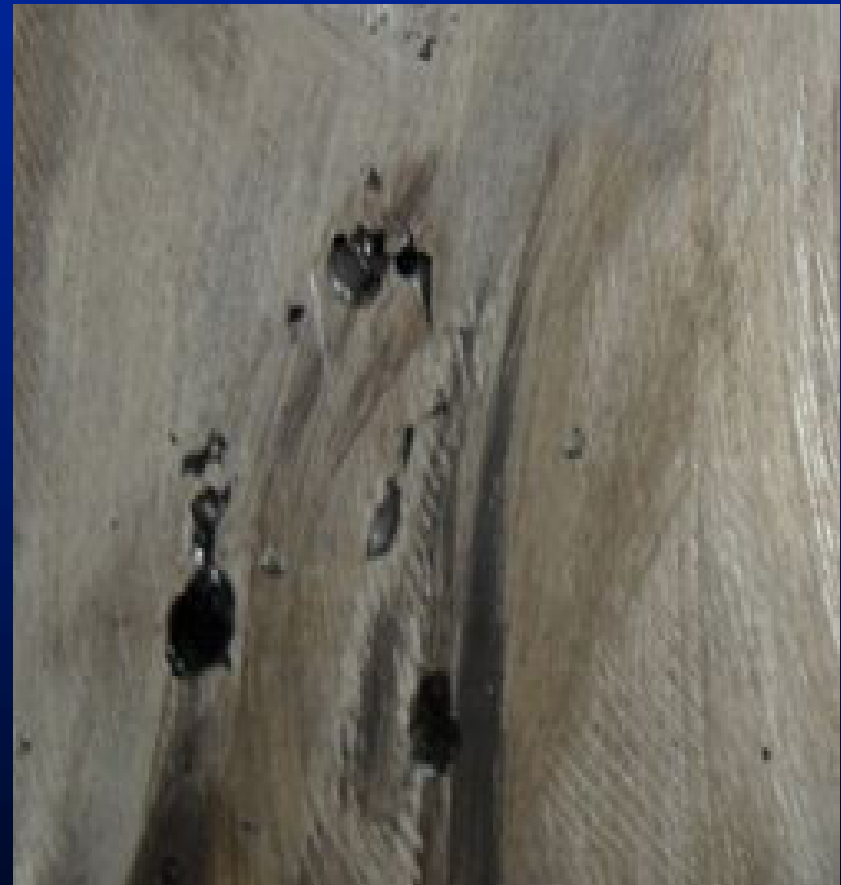
Sand Inclusion Defect
