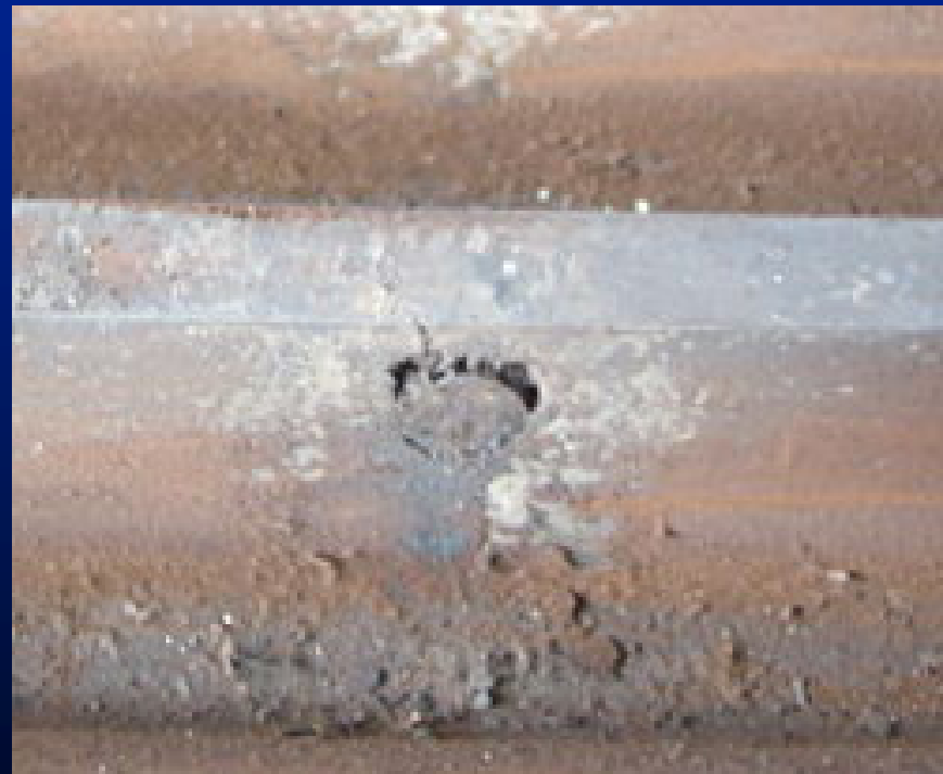
Slag Inclusion Defect
