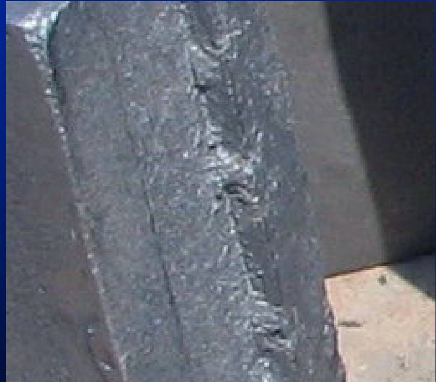
Sand Burning Defect
