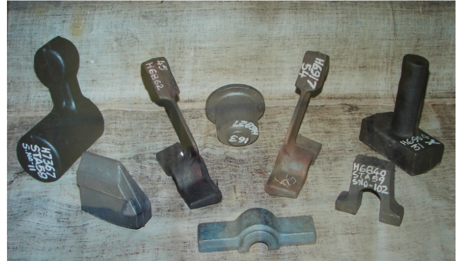
Closed die forged components
