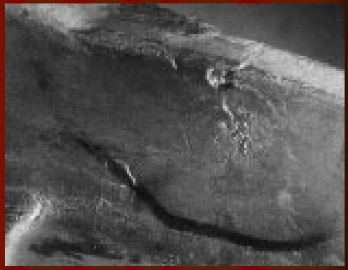
Surface defect occurs because it is always a race between the time of the molten metal arrives at a location in the die and the rapid solidification taking place.
