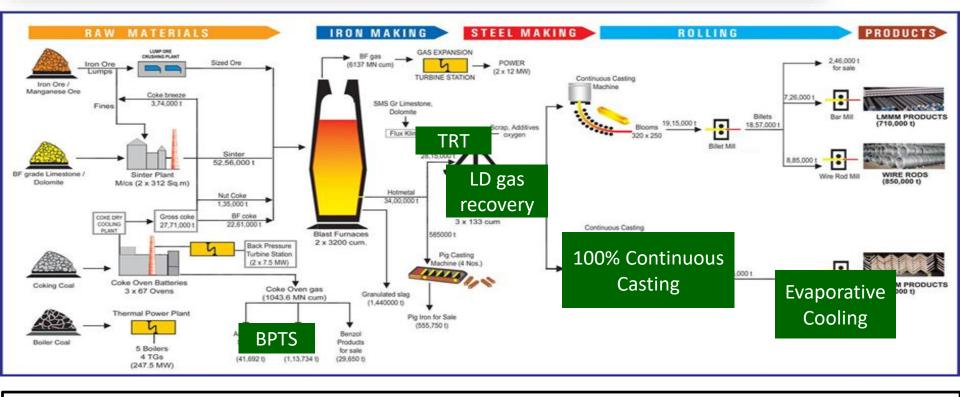
CO Battery with Coke Dry Quenching and Back Pressure Turbine Station 3200 cum BF with Top Recovery Turbine and BF gas recovery Rolling Mills with Stelmor & Tempcore (TMT) processes equipped with evaporative cooling for waste heat utilization
