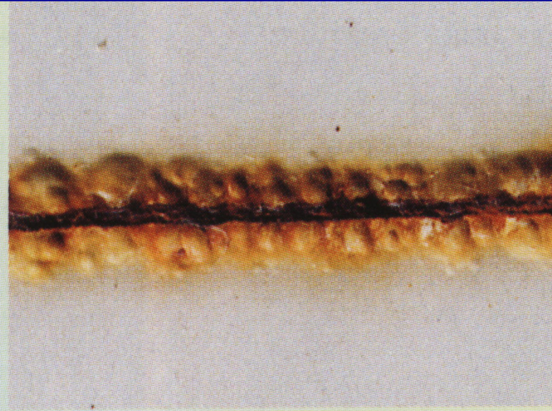
Painted steel sheet unprotected by zinc coating
