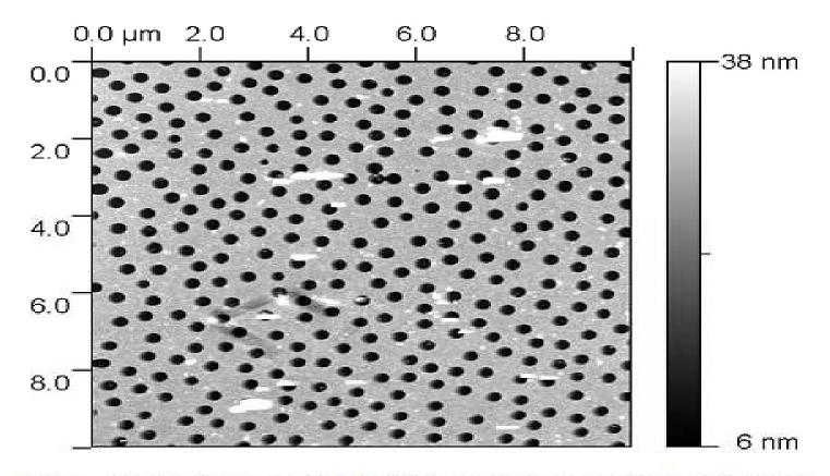
FIG. 1. Atomic force micrograph of 30-nm silver nanohole film fabricated by the colloidal lithography method using 350-nm latex spheres.
