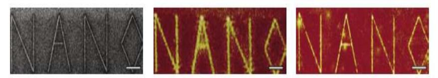
THIN LAYER OF SILVER acts like a superiens over very short distances. Here the word "NANO" is imaged with a focused ion beam (*left*), optically without a superiens (*middle*) and optically with
