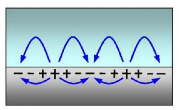
**FIGURE 1** Surface plasmon–polariton (SPP) propagating along a metal– dielectric interface. These waves are transverse magnetic (TM) in nature. Their electromagnetic field intensity is highest at the surface and decays exponentially away from the interface
