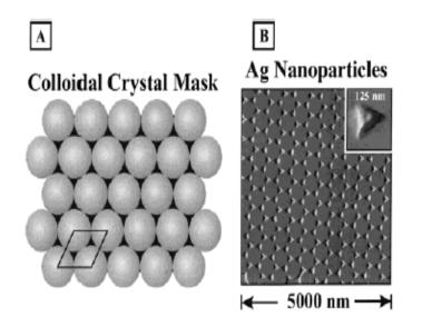
**Figure 1.** Schematic illustration (A) and representative AFM image (B) of SL PPA. The ambient contact mode AFM image was captured from a SL PPA fabricated with D = 542 nm nanospheres and  $d_m = 48$  nm thermally evaporated Ag metal after 3 min sonication in methylene chloride.
