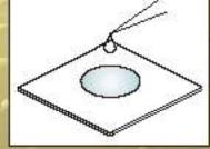
2. Dry in oven, spheres self-assemble at meniscus edge
