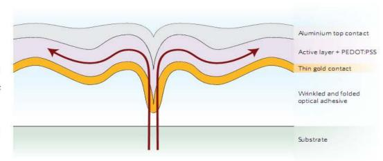
Figure 1 | Long-wavelength photons propagating across a wrinkled and folded substrate. Photons incident on the substrate side get 'folded' into the active layer of the cell by the folds in the polymer adhesive. The wrinkles further localize the light inside the layer through waveguiding effects. PEDOT:PSS, poly(3,4-ethylenedioxythiophene) poly(styrenesulphonate).
