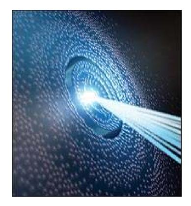
LIGHT BEAM striking a metal surface can generate plasmons, <u>electron density waves that can carry</u> <u>huge amounts of data.</u> If focused on a surface etched with a circular groove, as in this artist's rendering, the beam produces concentric waves, organizing the electrons into high- and low-density rings.
