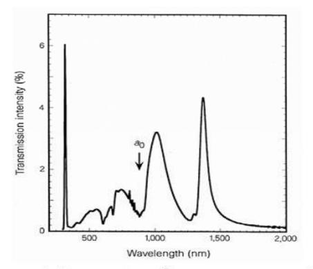
Zero-order transmission spectrum for a square array of 150 nm holes with a period of 900 nm in a 200 nm thick Ag film. The maximum transmitted intensity occurs at 1370 nm, nearly ten times the diameter of an individual hole in the array (Ebbesen 1998).
