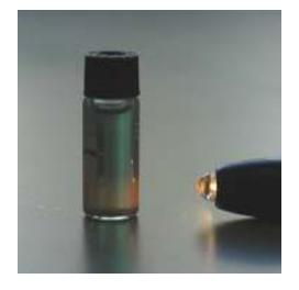
Au shell colloids in water (larger, also scattering)
