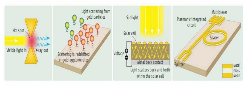
Applied plasmonics. (Left) A plasmonic hot spot between metal nanoparticles creates soft x-rays. (Middle left) Measuring the resonance shift in coupled metal nanoparticles leads to efficient sensing. (Middle right) Scattering from
