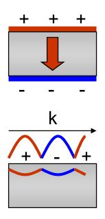
Plasmons in the bulk oscillate at  $\omega_{p}$ determined by the free electron density and effective mass
