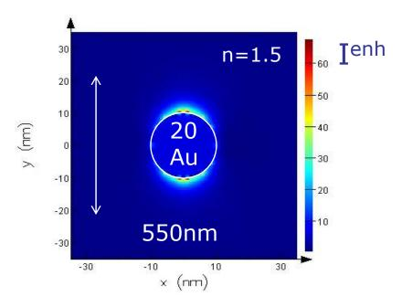
At resonance, both scattering and absorption are large
