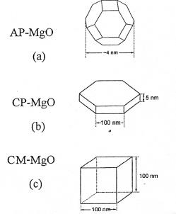
Models of (a) nanocrystalline (AP-MgO); (b) microcrystalline (CP-MgO); (c) normal commercially available (CM-MgO) magnesium oxide crystals. Reprinted with permission from *Clusters & Nanostructure Interfaces*, **1999**, p. 578, World Scientific Publishing Co Pte Ltd.<sup>1b</sup>
