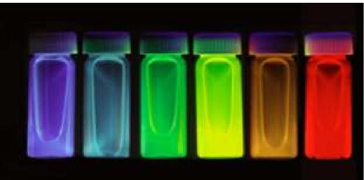
Colloidal CdSe quantum dots dispersed in hexane
