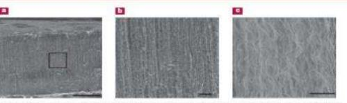
Structural characterization of macro tubes made from MWNT
