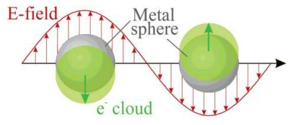
Figure: Schematic of plasmon oscillation for a sphere, showing the displacement of the conduction electron charge cloud relative to the nuclei.
