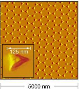
(a) Illustration of the process of **nanosphere lithography** (NSL) in which nanospheres are drop coated onto a surface and allowed to self-assemble into a hexagonally close-packed array (steps 1–3), followed by metal deposition (step 4), and (optional) removal of the nanosphere mask. (b) Atomic-forcemicroscope image of an NSL-fabricated nanoparticle array in which the nanosphere mask has been removed.
